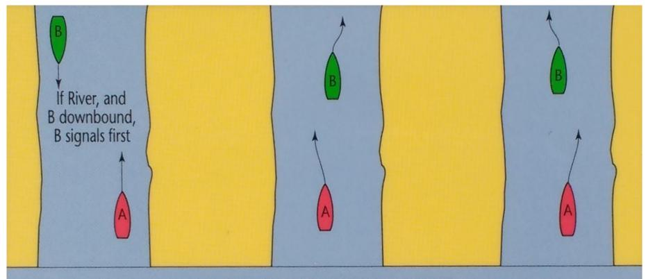
Meeting in narrow channel, both keep to starboard side of channel
